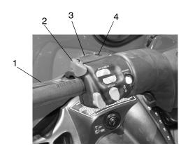
**NOTE:** If the brake lever is squeezed tightly enough, the lock will move freely into place. Do not force the lock or it may break.
